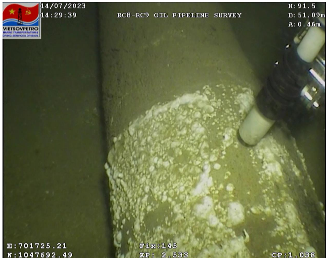
Figure 20: Anode CP reading: -1037mV at KP 2.532
