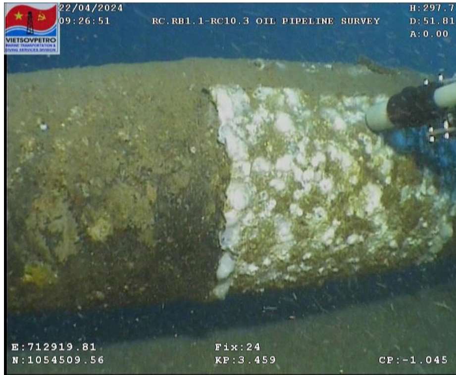
Figure 22: CP stab at Fix.24
