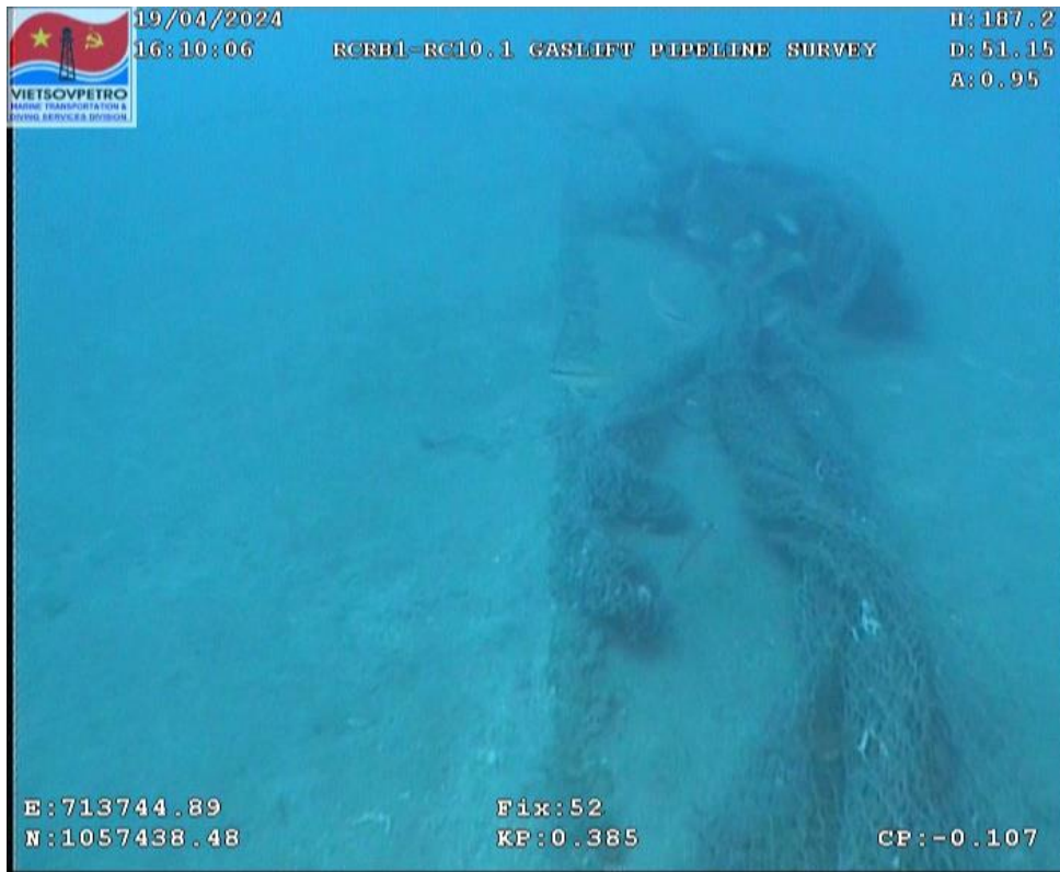
Figure 27: Debris soft netting at Fix .52
