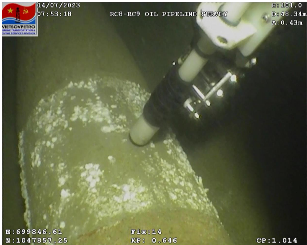
Figure 19: Anode CP reading: -1014mV at KP 0.647
