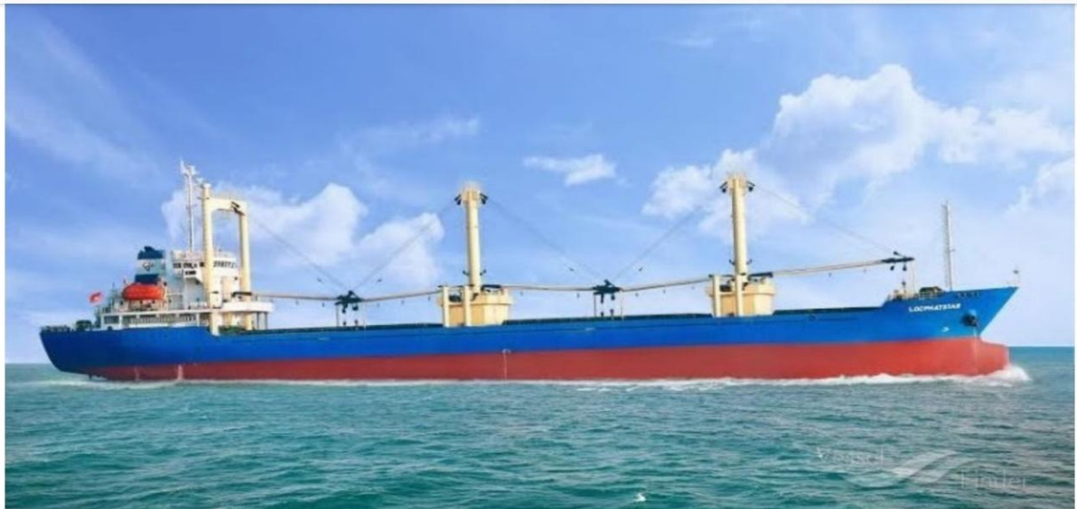
Vessel/barge with hydraulic crane or electric crane. The crane can rotate 360 0 and can be raised or lowered
