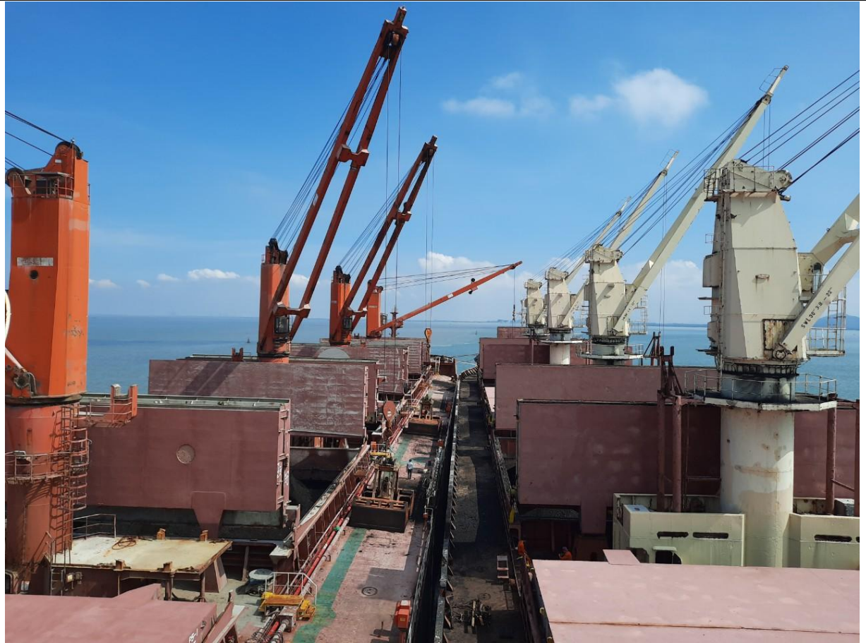
Vessel/barge with hydraulic crane or electric crane. The crane can rotate 360 0 and can be raised or lowered
