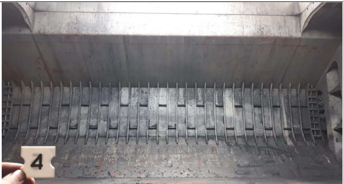
Vessel/barge with vertical keel being exposed but not extended to the bottom of the cargo hold, horizontal keel being not dragged along the cargo hold. The bottom of the cargo hold is flat;
