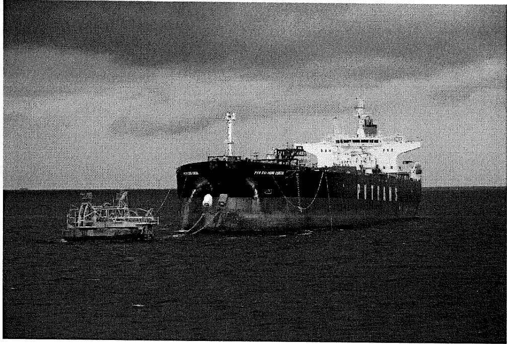
FSO is mooring to CALM buoy
