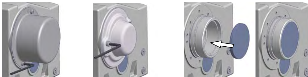
Figure 3-12: Fitting the covers, Option SH, Option H, and Option H66
